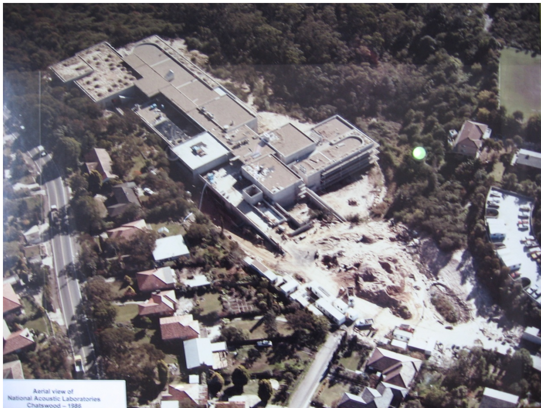
Figure 8 - 1986 Aerial photographs of the site showing the constructed National Acoustic Laboratory and Ultrasonics Institute and decked parking structure. The second photograph shows the extensive earthworks that occurred around the minor tributary of the Blue Gum Creek
